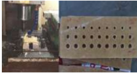
Fig. 3 Final Test specimen after drilling
